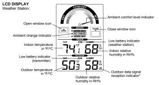
\* When the signal is successfully received by the wireless weather station, the outdoor transmission icon will be switched on. (If not successful, the icon will not be shown on LCD). The user can then easily see whether the last reception was successful (icon on) or not (icon off).
